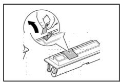
Install the new *Toner Container* in the printer. Push firmly on the top of the container at the positions marked PUSH HERE, until you hear a click.
